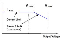
The power limit (maximum continuous power) is due to the converter's heat dissipation capacity
